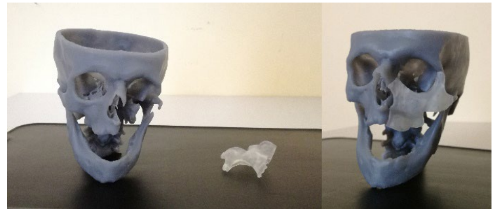
Izrada lubanje i implantata korištenjem 3D printera Form 2 – konačan model / Making skull and implant using 3D printer Form 2 – the ultimate model
