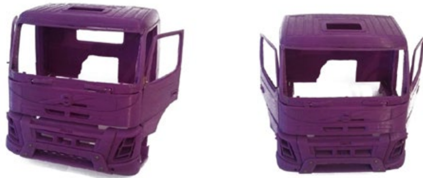
Model kabine napravljen na 3D printerom / A cabin model compiled on a 3D printer
