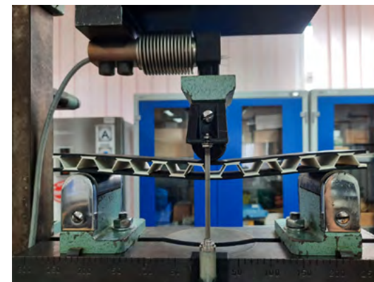
Kompozitna sendvič struktura PLA-ABS-PLA s trapeznom jezgrom prije i nakon spajanja / Composite sandwich structure PLA-ABS-PLA with trapezoidal core before and after joining
