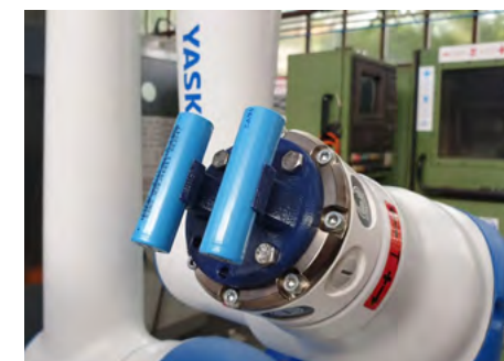
3D ispisana hvataljka za 18650 litij-ionske baterije montirana na robotskoj ruci YASKAWA HC10DT / 3D printed gripper for 18650 lithium-ion batteries mounted on a YASKAWA HC10DT robotic arm
