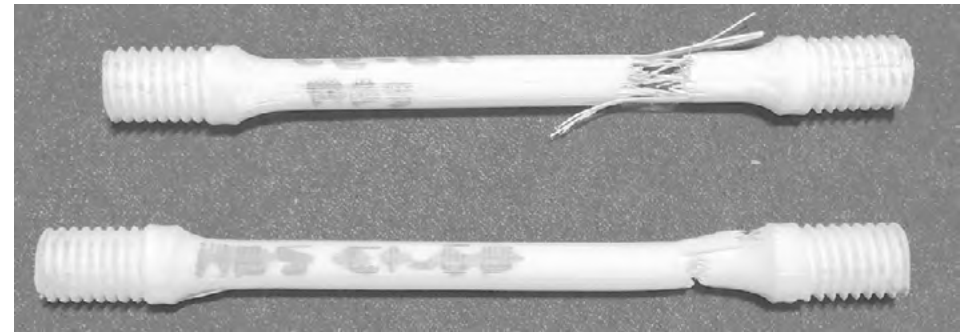
ABS testne epruvete nakon eksperimenta puzanja konstantne temperature T = 50^\circ\text{C} . / ABS test-tubes after the creep experiment at constant temperature T = 50^\circ\text{C} .
